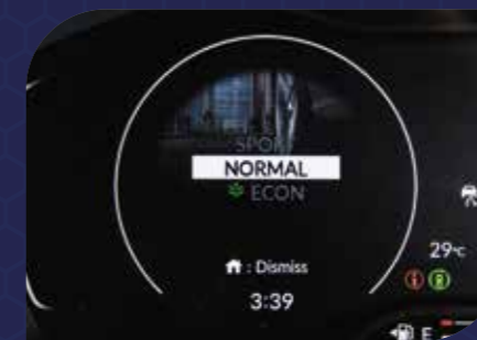
3 Drive Modes (Normal, Sport, Econ) Toggle between Normal mode for relaxed street driving, Sport mode for sharpened response and heightened enjoyment, and Econ mode to optimise fuel efficiency.
